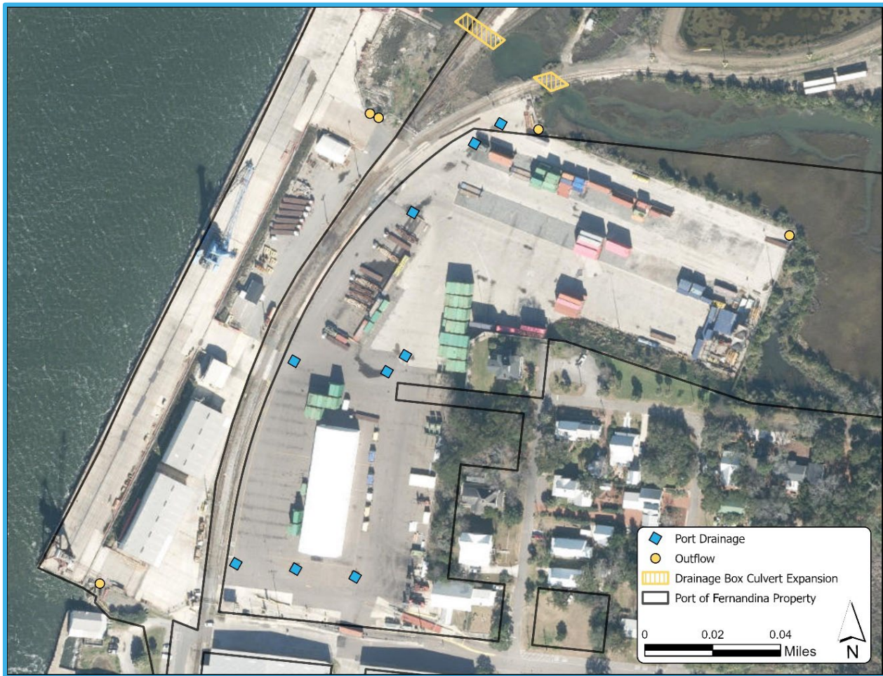
Figure 29 - Improved Drainage and Water Management System
