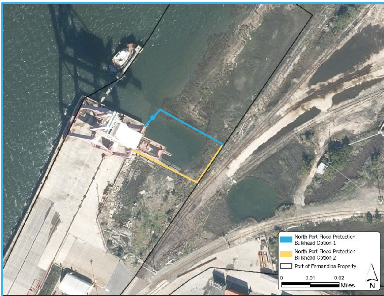
Figure 24 - North Port Flood Protection Bulkheads
